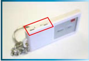
The switch to select the mode the sensor operates in can be found on the side of the remote control, as shown to the left.
