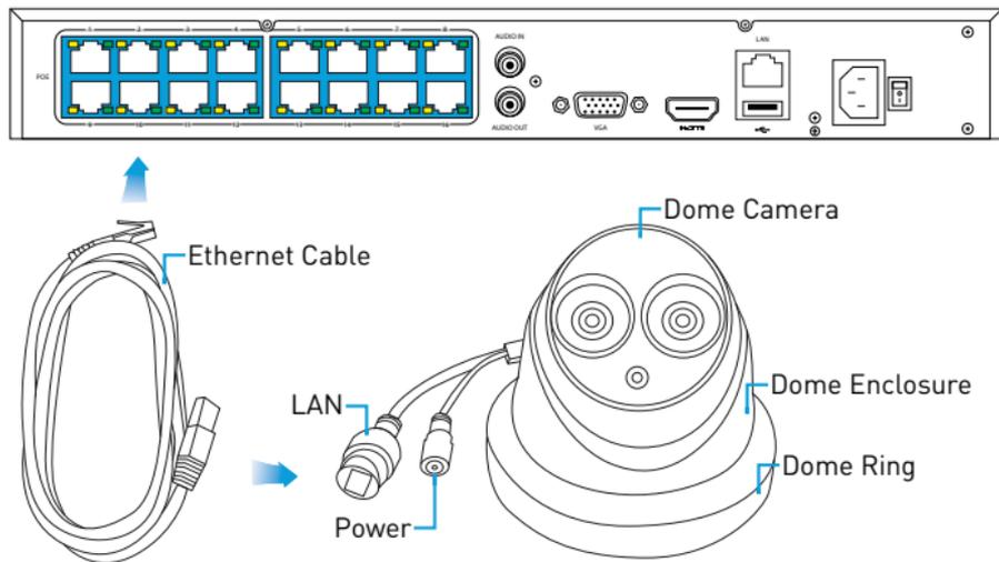
The Ethernet cable is the same at both ends so it doesn't matter which end plugs into the camera or the NVR. For more information on how to configure your camera, please consult the user guides included with your NVR.
