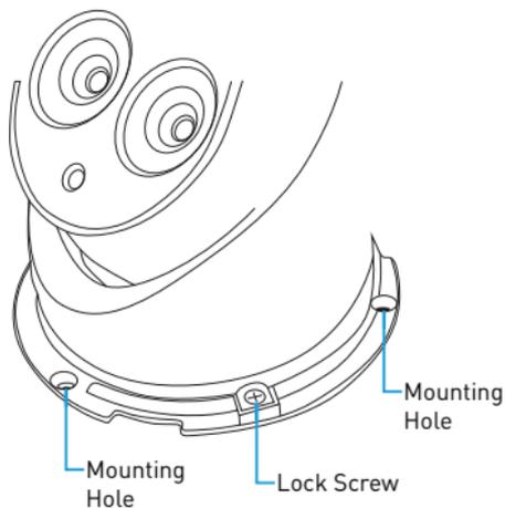
The camera can be mounted onto a flat vertical or horizontal surface and must be of sufficient strength to hold the camera -
