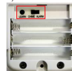
Inside the Battery Compartment showing the Mode Switch and LEARN button.
